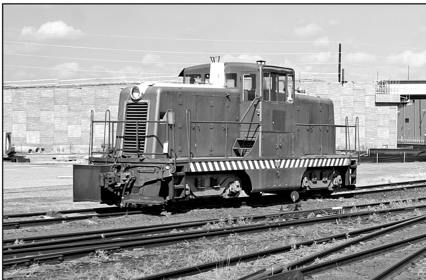
The seldom-used Cargill switcher is near the nearly complete Pecos Street overpass at the west end of the Union Pacific (was Rio Grande) North Yard in Denver on July 2, 2011. This 65-ton diesel was built in 1943, and has been replaced here by a modern Shuttle Wagon railcar mover. – Photo © 2011 Dave Schaaf.
